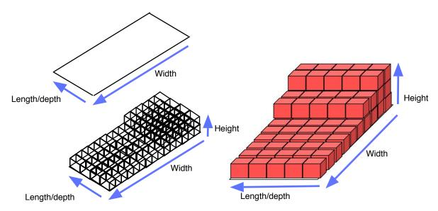
By combining these two steps (area of the bottom of the object and height of the object), we can find the volume of a regularly-shaped object. The area of the bottom (length x width) times the height of the object or  $L \times W \times H$  equals the volume of the object.
