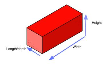
Let's focus first on the bottom or base of the box. Note that by multiplying the length by the width of the bottom of the object, we can get the area of the bottom of the object. In Lesson 2 we referred to these two measurements as the length and height of the shape. Let's rename "height" to "width" to reduce confusion.
