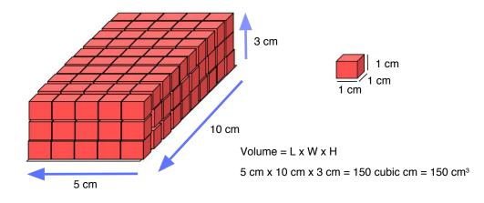
In this example we used centimeters as our units of length. We have the length in cm x width in cm and the height in cm. Multiplying these together we get cm<sup>3</sup> or cubic centimeters. So, our volume measurement is in cubic units. An object measured in inches would have a volume in cubic inches; in feet, the volume would be in cubic feet. Something very large might have its volume measured in cubic miles. The key here is that volume is measured in cubic units.
